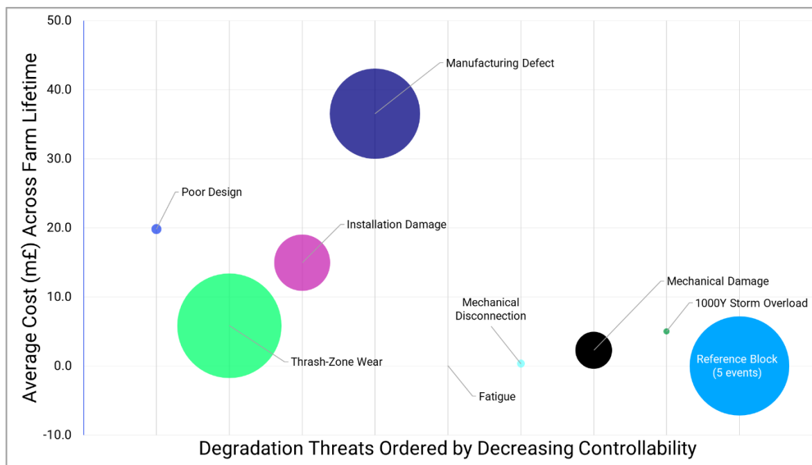
Figure 2: Cost and occurrence of degradation threats across a 50-unit farm.
