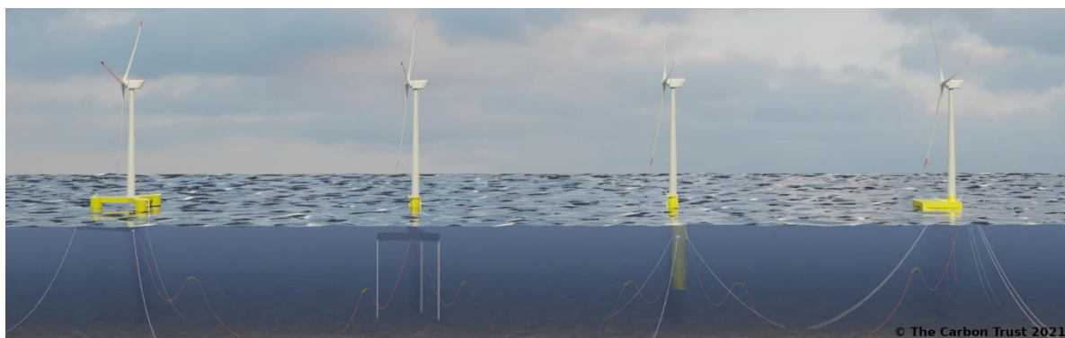
Figure 1: 15 MW reference substructure designs for the Floating Wind JIP. This project was based upon an updated version of the semi-submersible design.
